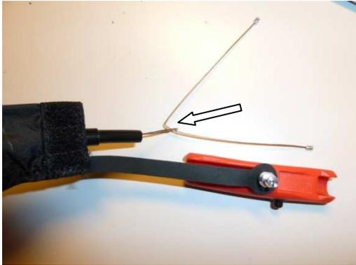
**Step 9:** Pass the two extremity of the new cable inside the slit on the metallic part of the handle. (The two extremities must pass on the same side)
