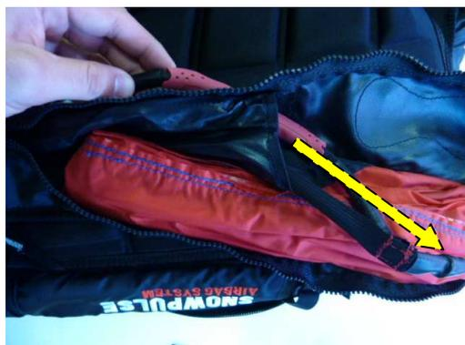
**Step 4:** Cut the black thermo hose, without cutting the strap behind; you can then see the handle extremity
