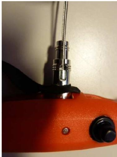
**Step 10:** Push the hoses onto the metallic part until the metallic part is fully covered. You have to slide the small diameter then the bigger one.
