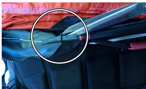
**Step 5:** Cut the handle strap without arming the cable. Remove any part of the old strap
