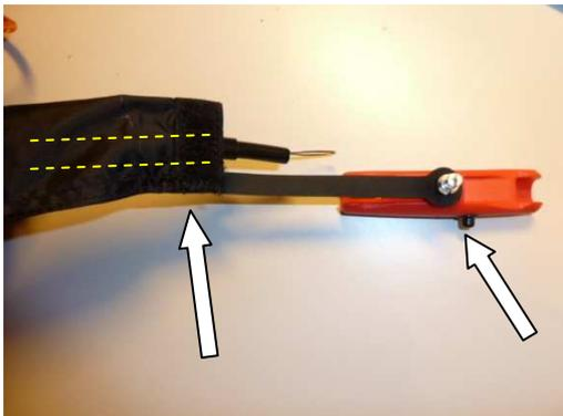
**Step 8:** Pass the new short cable inside the loop of the other one
